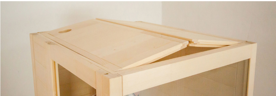
Fig. 15: Fastening the ceiling elements
