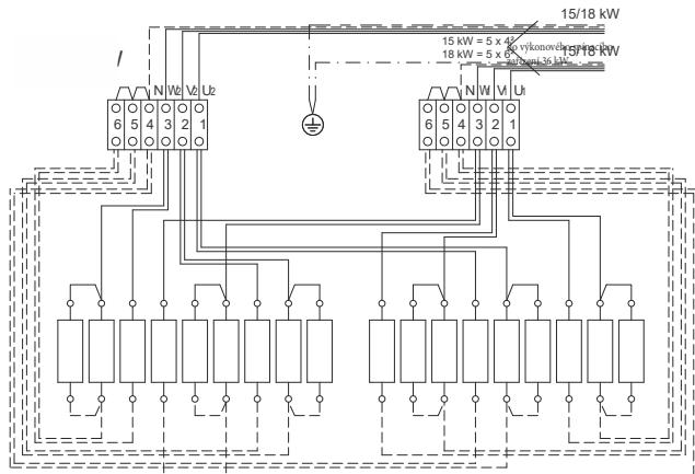
$$30 \text{ kW} = 18 \times 1,666 \text{ kW}$$
